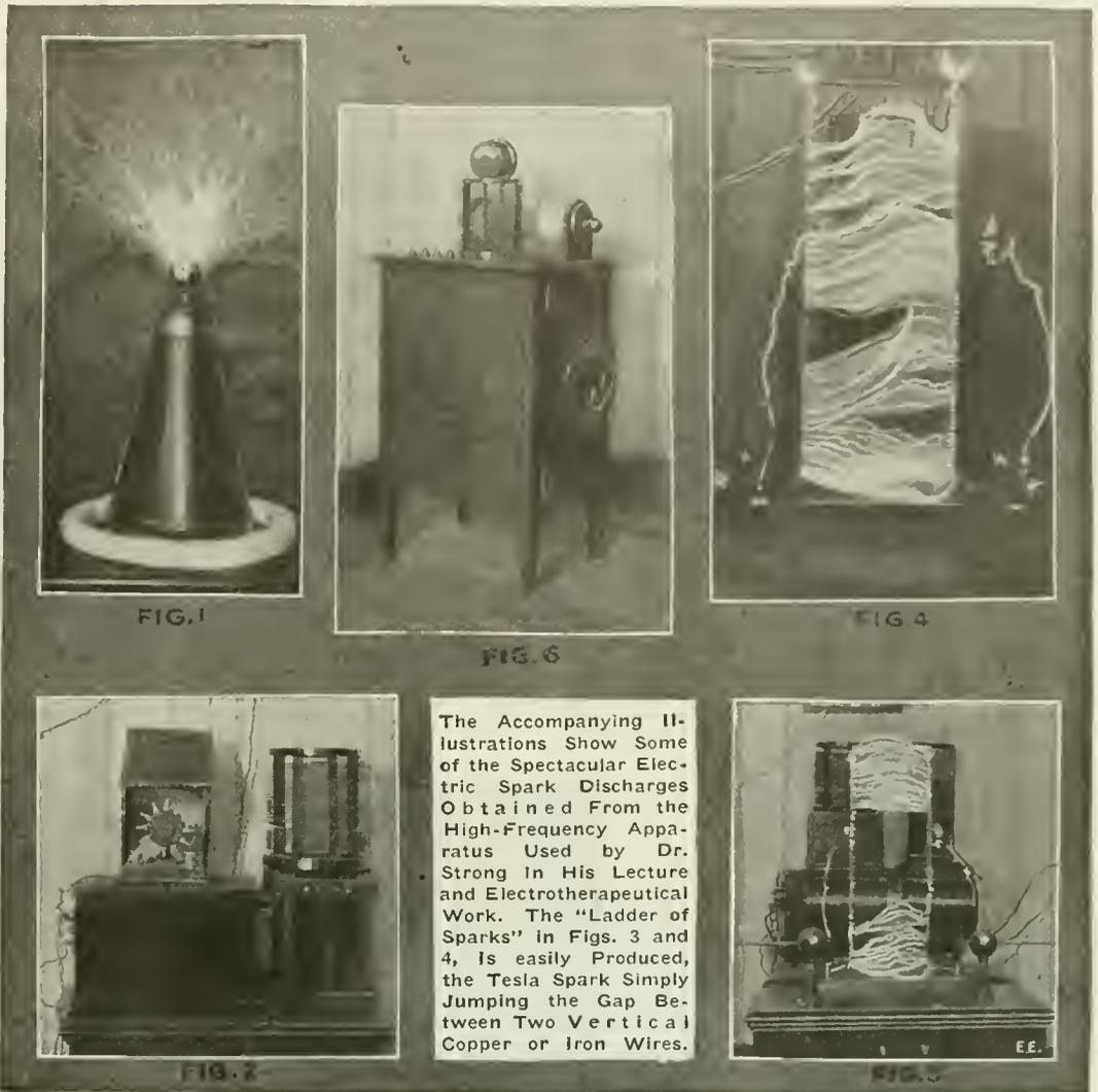
The Accompanying Illustrations Show Some of the Spectacular Electric Spark Discharges Obtained From the High-Frequency Apparatus Used by Dr. Strong In His Lecture and Electrotherapeutical Work. The "Ladder of Sparks" in Figs. 3 and 4, is easily Produced, the Tesla Spark Simply Jumping the Gap Between Two Vertical Copper or Iron Wires.
