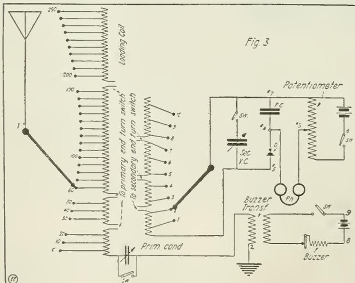
Hook-Up for Complete "Marconi" Type 106 Receiving Set, Showing Inductively Coupled Test Buzzer.
