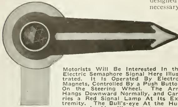
Motorists Will Be Interested In the Electric Semaphore Signal Here Illustrated. It Is Operated By Electro-Magnets, Controlled By a Push Button On the Steering Wheel. The Arm Hangs Downward Normally, and Carries a Red Signal Lamp At Its Extremity. The Bull's-eye At the Hub Is Also Illuminated.
