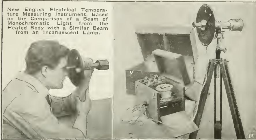
New English Electrical Temperature Measuring Instrument, Based on the Comparison of a Beam of Monochromatic Light from the Heated Body with a Similar Beam from an Incandescent Lamp.
