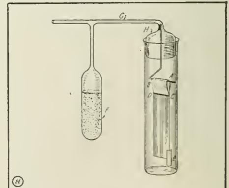
Arrangement of Apparatus for Measuring Pressure of Light.—H is Hollow Stopper, E is Cover Glass Cemented to Tube, F Contains Pith Charcoal, G is Tube Which May Be Connected to Gauge Pump.
