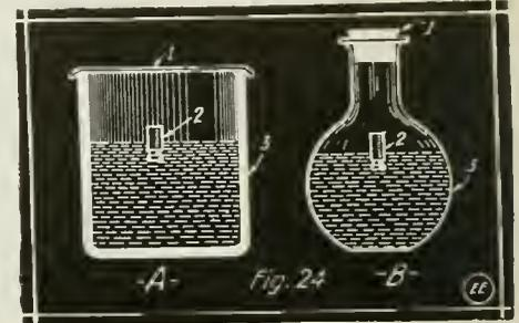
Apparatus With Which the Principle of the Submarine Can Be Demonstrated. The Small Vial 2, Can Be Made to Perform Many Wonderful Tricks By Pushing Down on Diaphragm 1, or Squeezing Bottle 3 in "B".
