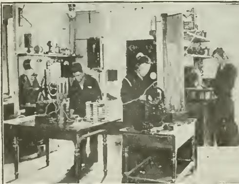
Future Naval Radio Men Learning How to Measure Length and Frequency of Etheric Waves.
