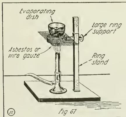
Correct Manner in Which to Place "Evaporating Dish," Wire Gauze and Bunsen Burner.
