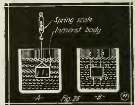
Proving the "Law of Buoyancy," *i. e.*, That Objects Weigh Less In Water Than In Air.
