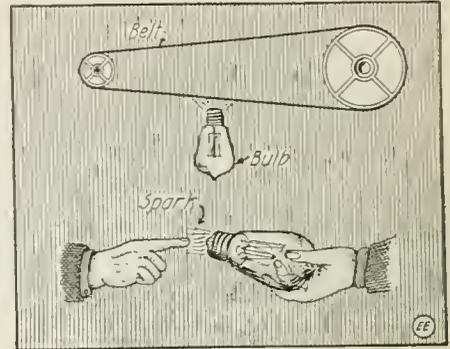
Hold an Incandescent Lamp Bulb Near a Rapidly Moving Belt—Usually Sufficient Static Electricity Will Pass to Charge the Lamp as a Condenser. It Will Give Powerful Shocks.
