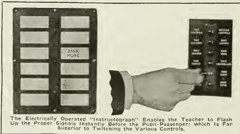
The Electrically Operated "Instructograph" Enables the Teacher to Flash Up the Proper Signals Instantly Before the Pupil-Passenger; which Is Far Superior to Twitching the Various Controls.
