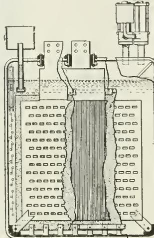
is caused to flow there-thru from one electrode to another, both electrodes being submerged in water. The solution is decomposed in the well-known electrolytic manner, oxygen being liberated at the positive electrode and hydrogen at the negative electrode. This invention relates particularly to an electrolytic gas generator in which the liquid acted upon is contained in a suitable receptacle, having two sets of insulated electrodes entirely independent of the receptacle proper.
