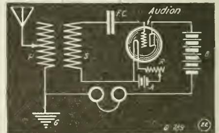
Hook-up for a Short Wave Regenerative Audion Radio Receiver.
