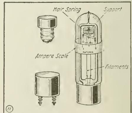
By Placing the Delicate Moving Parts of This High Frequency Current Gage in an Evacuated Bulb the Action is Made More Stable and Reliable. It Can Be Used with a Wave Meter to Measure the "Decrement."
