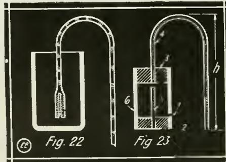
Two Forms of Automatic Siphon. Details for Constructing the One on the Right Are Given Herein.
