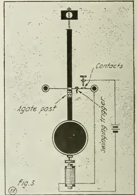
Finally the Electric Clock Problem Settled Down to a Resurrection of Hipp's Famous Pendulum. But Oh! that "Agate" Post! X? Likewise Zowie.
