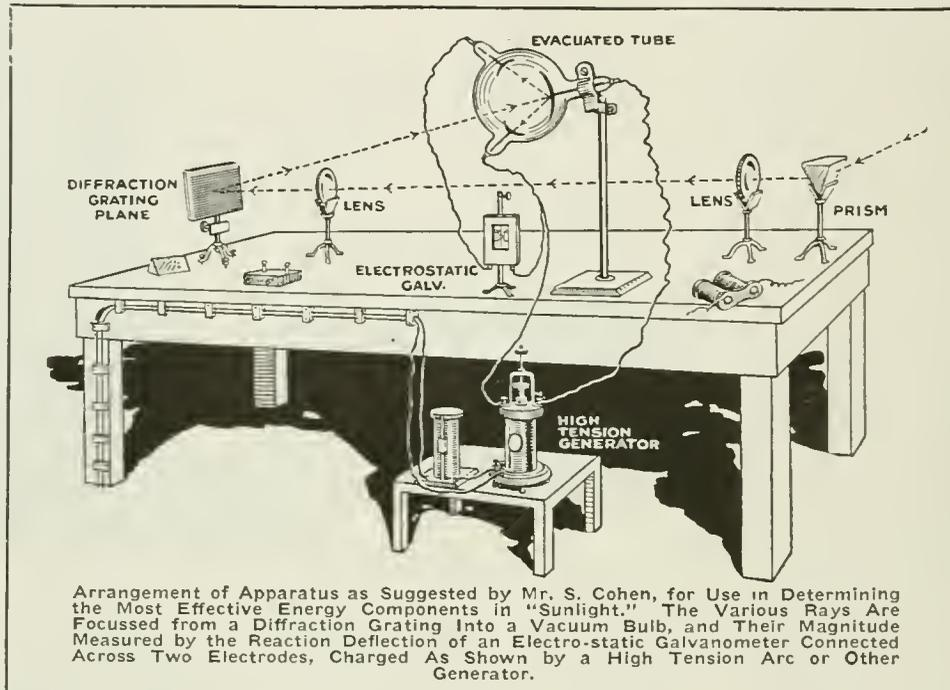
Arrangement of Apparatus as Suggested by Mr. S. Cohen, for Use in Determining the Most Effective Energy Components in "Sunlight." The Various Rays Are Focused from a Diffraction Grating into a Vacuum Bulb, and Their Magnitude Measured by the Reaction Deflection of an Electro-static Galvanometer Connected Across Two Electrodes, Charged As Shown by a High Tension Arc or Other Generator.
