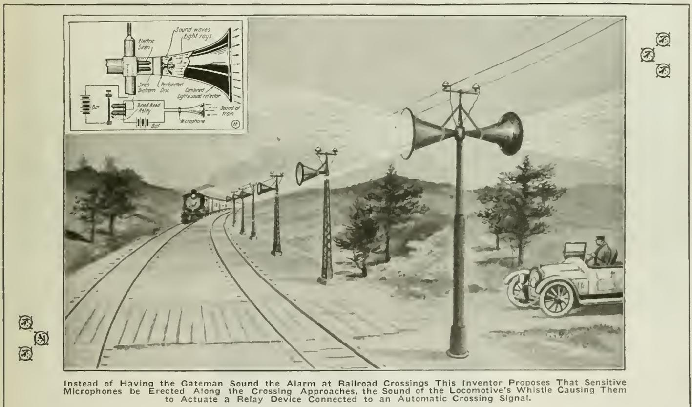
Instead of Having the Gateman Sound the Alarm at Railroad Crossings This Inventor Proposes That Sensitive Microphones be Erected Along the Crossing Approaches, the Sound of the Locomotive's Whistle Causing Them to Actuate a Relay Device Connected to an Automatic Crossing Signal.
